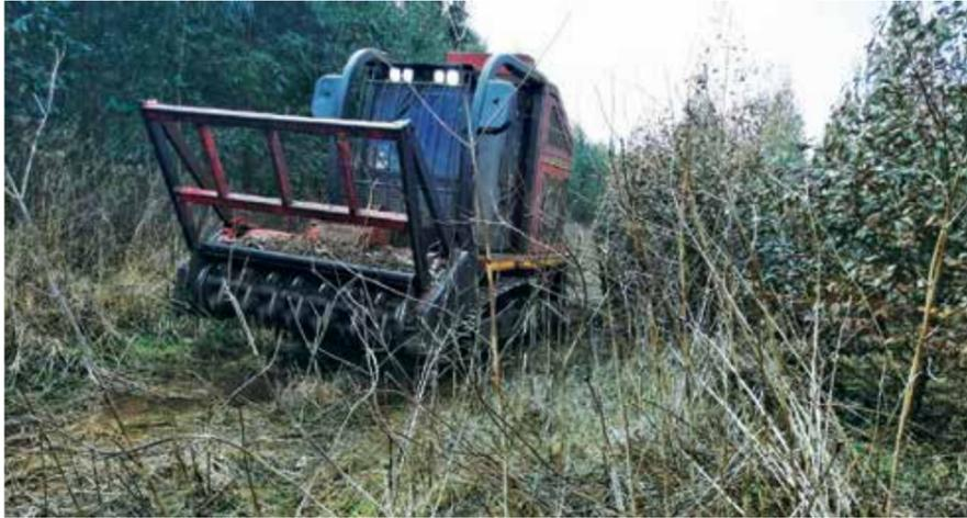
Inter-row mulching with the RT 200 reduced fuel loads (stumps and slash) and improved access to the compartment.
